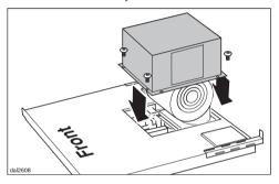
■ Mount the blower box to the housing with 4 screws.
